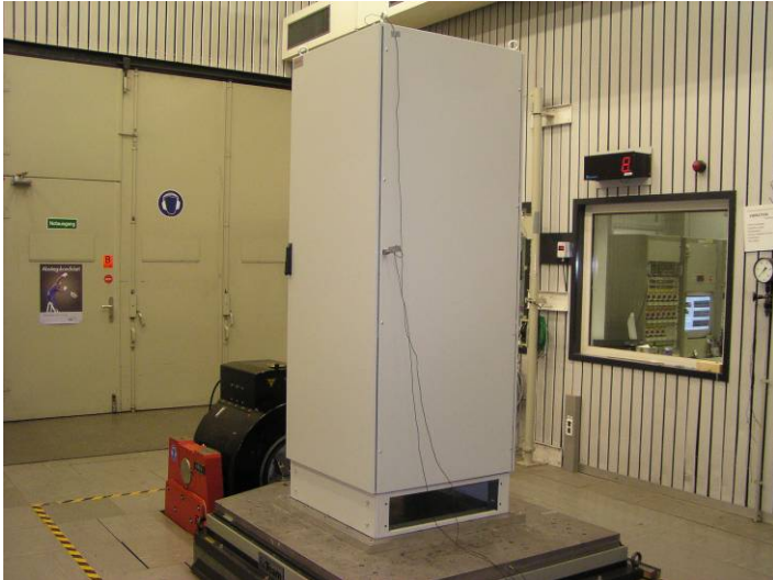
Pic. 6 Mounting of EUT for X-axis test
