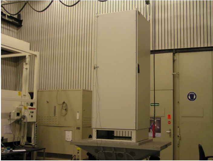
Pic. 5 Mounting of EUT for Z-axis test
