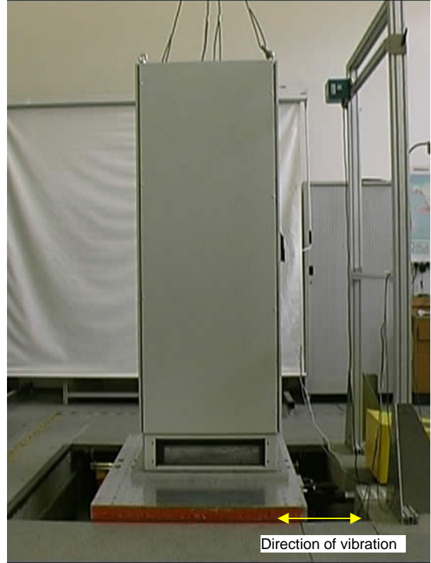
Pic. 13 Mounting of EUT for Y-axis test
