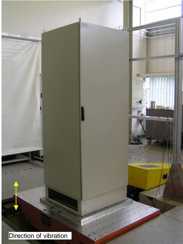
Pic. 12 Mounting of EUT for Z-axis test
