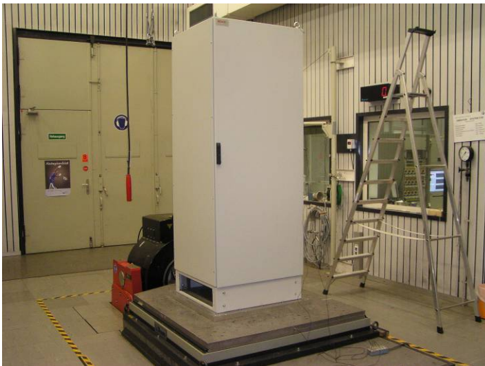
Pic. 7 Mounting of EUT for Y-axis test
