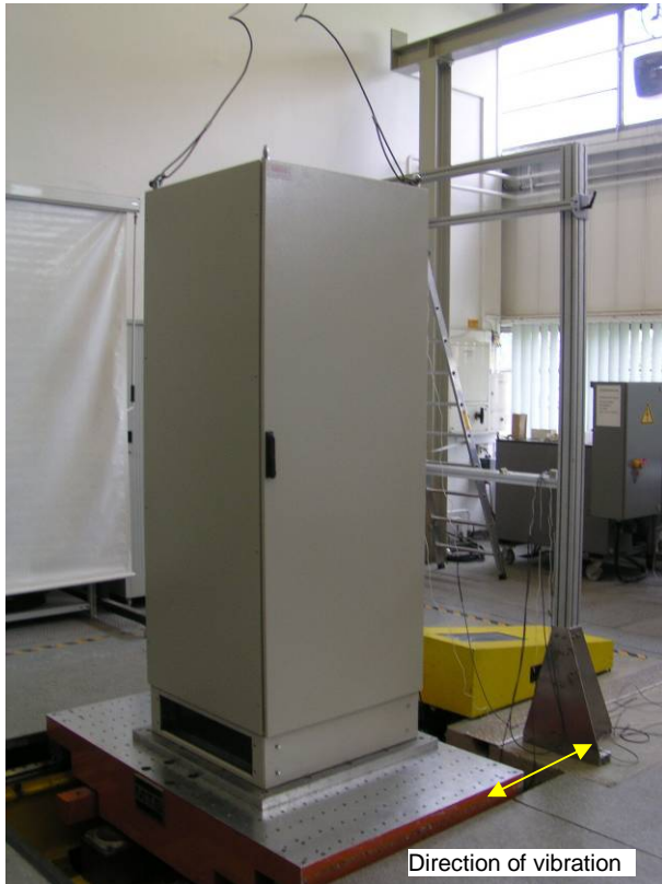
Pic. 14 Mounting of EUT for X-axis test
